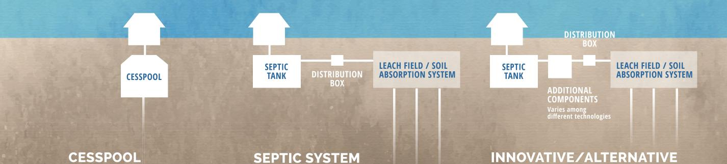
A cesspool is a pit which provides wastewater a place for both the solids to settle and also for liquid to disperse to the surrounding soil.
