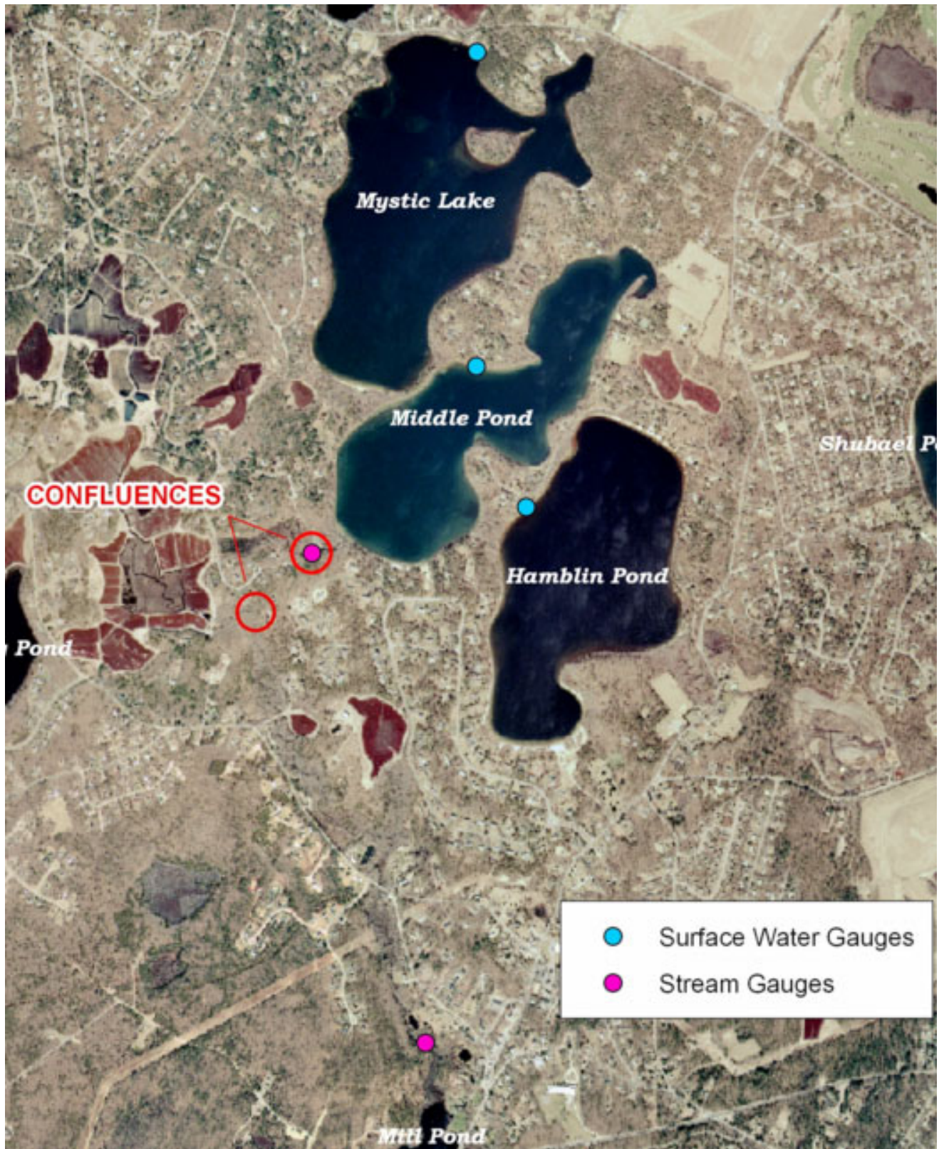
Figure 5. Stream and pond water level gauges in the Indian Pond study area.
